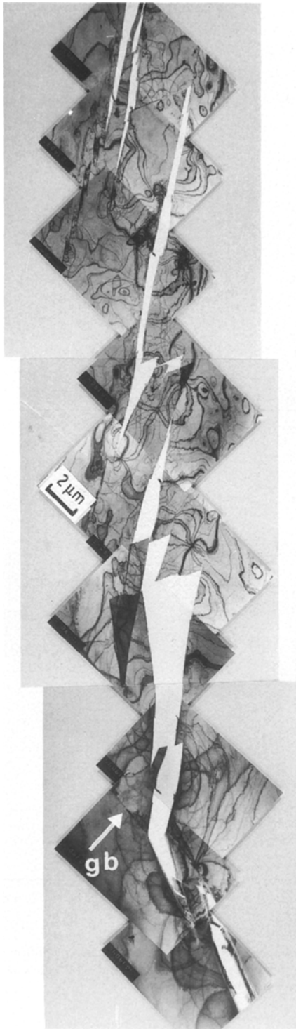
Figure 3 The same specimen as in Fig. 1 after straining. The zig-zag shaped crack propagation is characteristic of the material.
